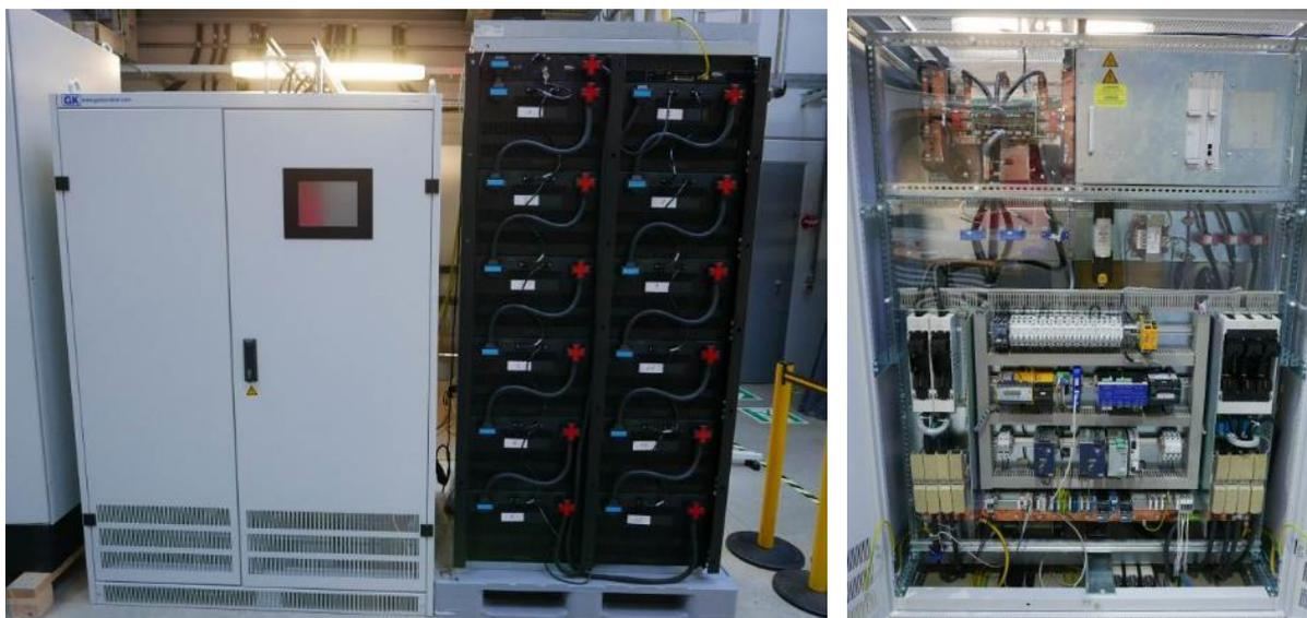
Figure 9: Central storage system for the field trial in Heimschuh setup in the AIT SmartEST Laboratory – full system (left) and inner setup of inverter (right)
