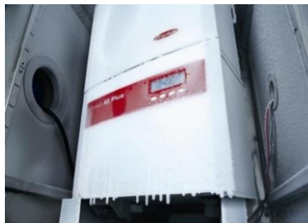
Figure 20 Inverter in climate chamber under freezing test
