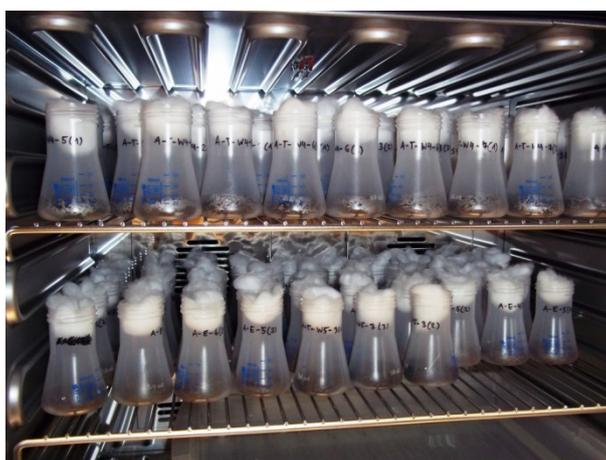
*Figure 19 Erlenmeyer flasks filled with soil-BC mixtures. The flasks are placed inside the incubator. The flasks were plugged with cotton balls to prevent contamination.*
