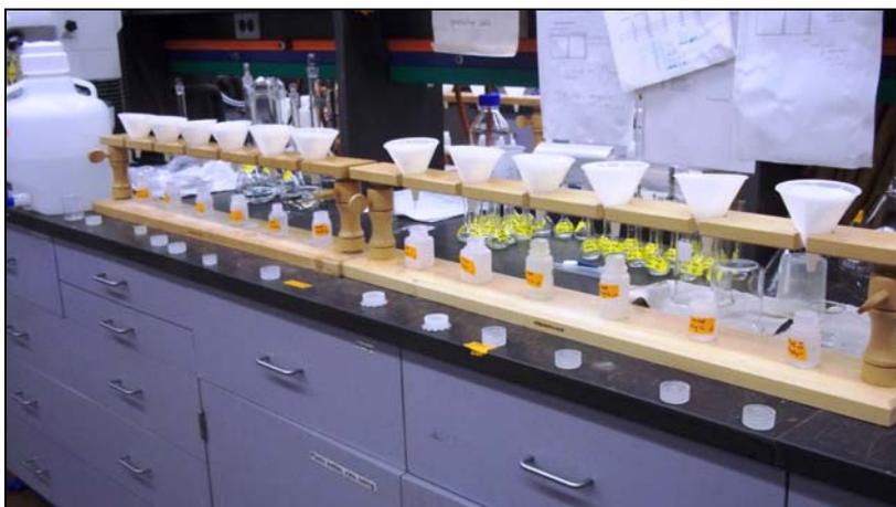
Figure 57 Filtration of samples after 24 h adsorption
