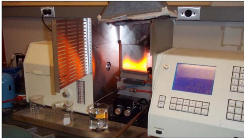
Figure 59 Atomic absorption spectrometer
