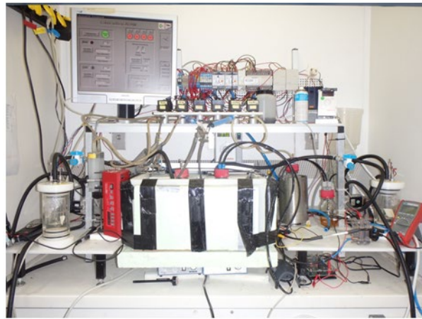
Figure 1: H 2 milking reactors. In the picture the first setup is shown, which included an experimental reactor and a control reactor.
