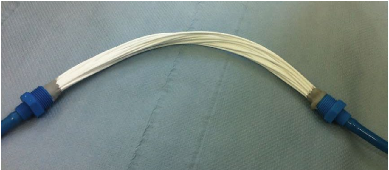
Figure 2: Small membrane module with 153 cm 2 membrane surface area.
