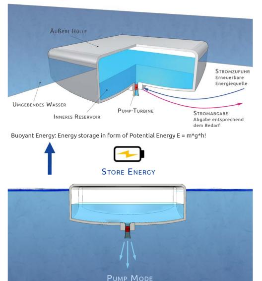
Buoyant Energy - Floating pumped-storage hydropower
