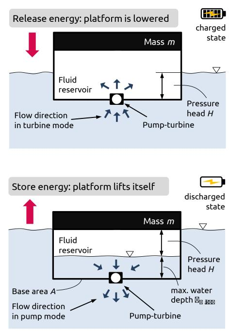
Energy storage and regulation becomes increasingly important in electrical networks with a growing share of renewable energies with fluctuating generator characteristic. Today, pumped-storage hydro-power (PSH) plants store electrical energy almost exclusively (over 99 % worldwide). When used onshore, this well-established technology has outstanding features, but is restricted to mountainous regions.
