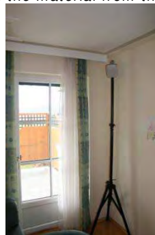
Setting up the Ubisense: tripods in open spaces and supports over furniture
