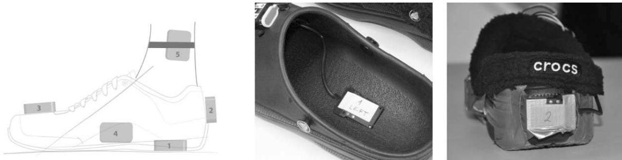
Image 1: Prototype of our wearable sensor device implemented as shoe, based on the Inertia Cube III
