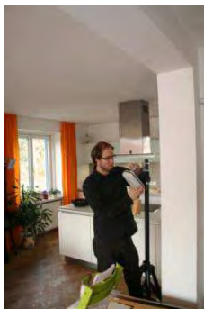
Setting up the Ubisense: tripods in open spaces and supports over furniture
