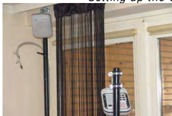
Setting up the Ubisense: tripods in open spaces and supports over furniture
