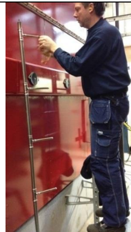
Figure 32: Suction pyrometer is used for the temperature measurements at four levels of the vertical shaft in the biomass furnace. The highest probe corresponds to the highest temperature, i.e. the first measuring point meeting the gas stream
