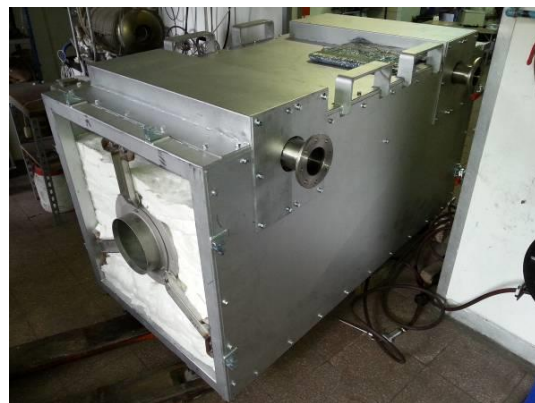
Figure 41: HT-HE with the ceramic insulation material (partial filling)
