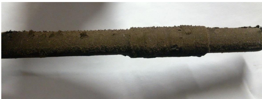
Figure 13: Probe with the four test rings after a few days of exposure
