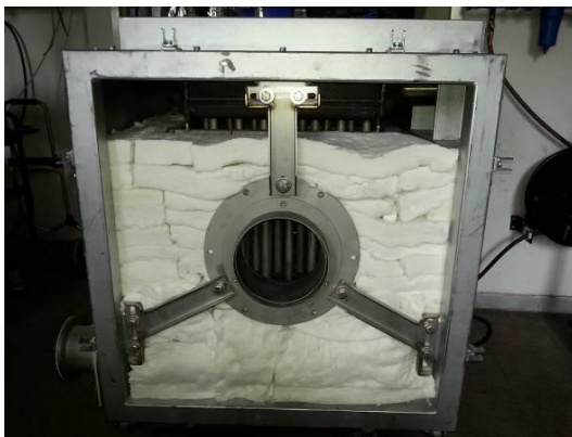
Figure 41: HT-HE with the ceramic insulation material (partial filling)
